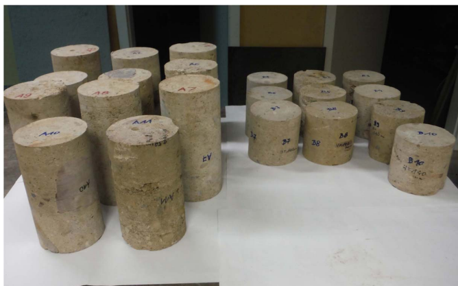
Fig. 1. Core sample Types A and B after cut geometry preparation.
